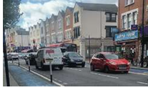
Lightly segregated cycleway.
