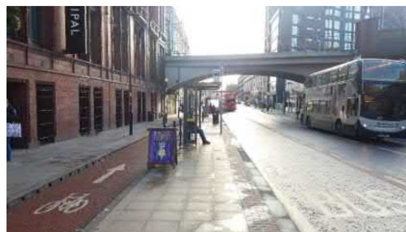
Figure 3.8. Segregated cycleway (carriageway height)
