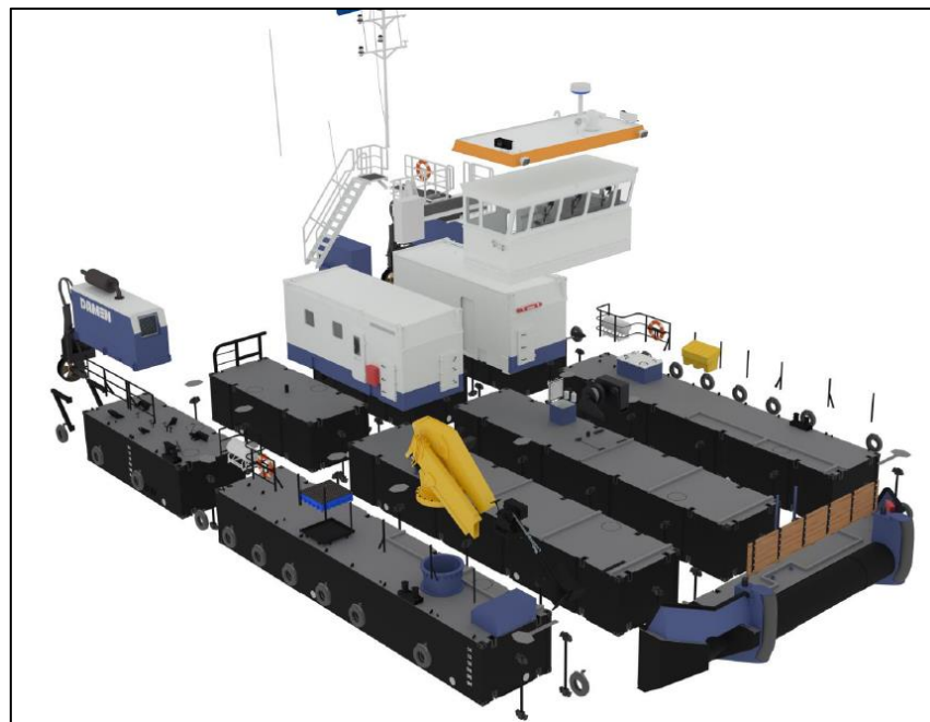
An example of a fully modular vessel design with modules that bolt together (Ref. E)
