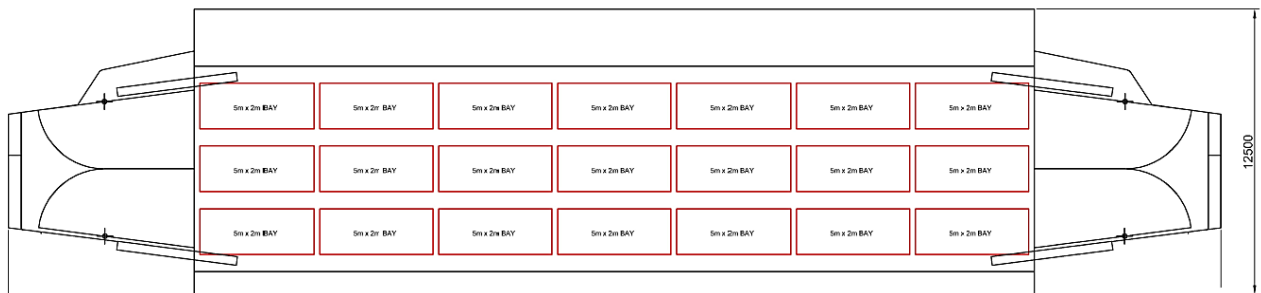
New ferry vehicle deck option with 21 cars in 3 lanes
