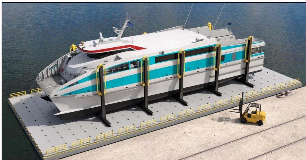
The TugDock road-transportable drydock system ( tugdock.com/ )
