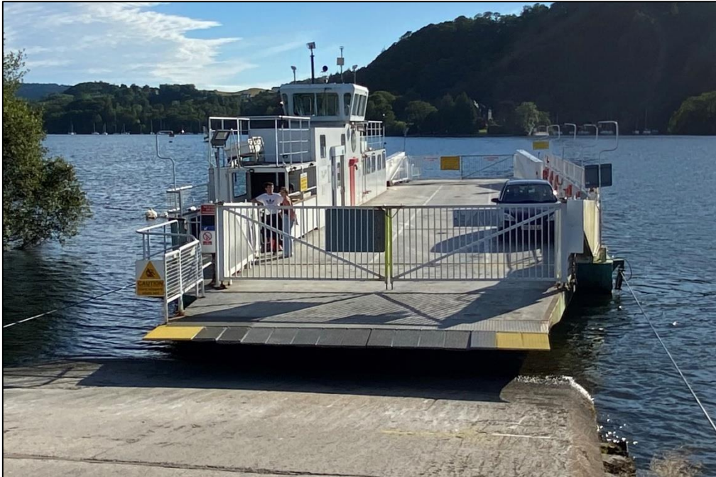
Mallard approaching the Ferry Nab (east) slipway, the two drive cables can be seen
