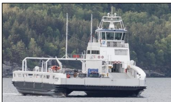
The 80m car ferry Ampere entered service in Norway in 2015 and carries 120 cars on a 20-minute crossing 34 times a day
