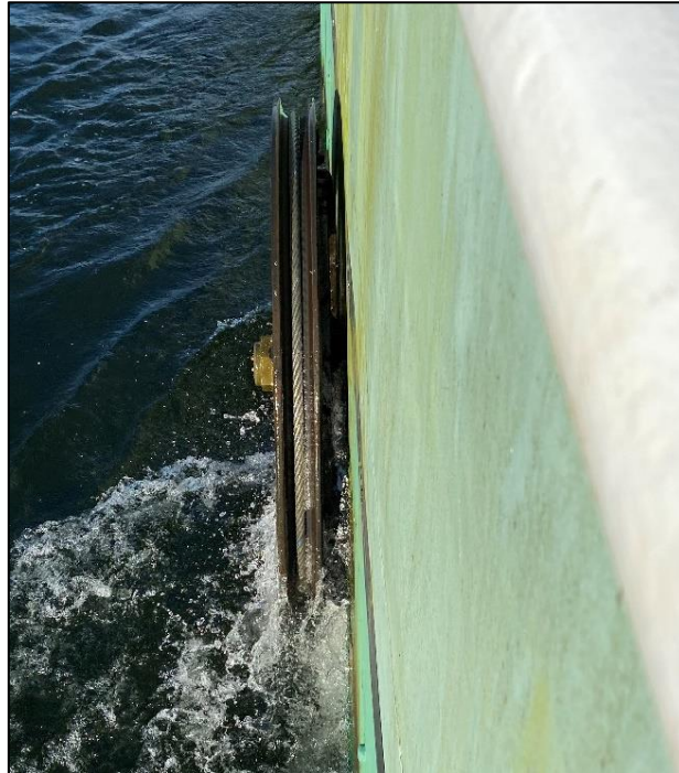
One of Mallard's cable drive wheels
